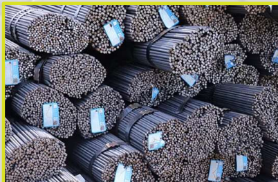
Bundled rebar with dunnage
